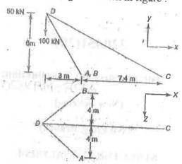
(c) Using tension coefficient method analyze the member forces in truss as shown in figure:
